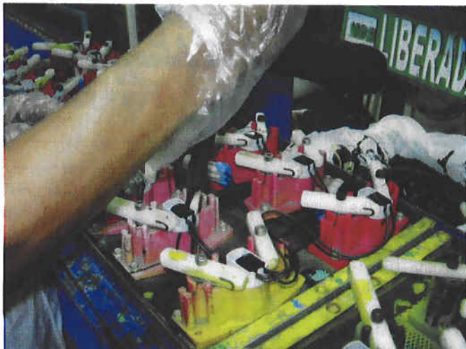
Empire has moved beyond doing just wire harness assembly. Socket potting (shown) is one example of the company's many in-house capabilities.
