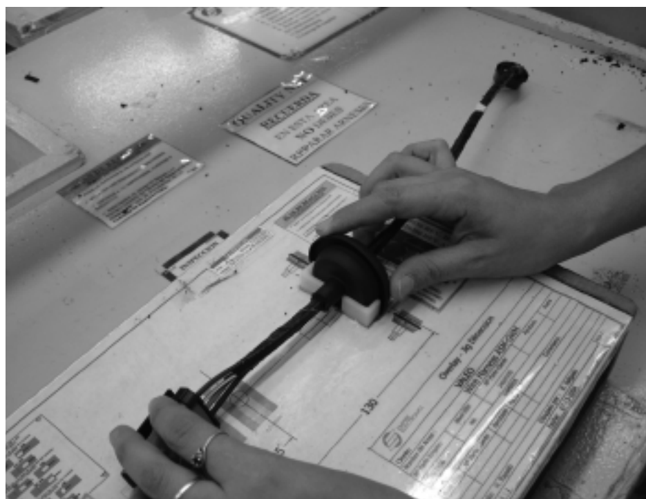
Dimension inspection is a critical aspect in the quality control of wiring harnesses.
