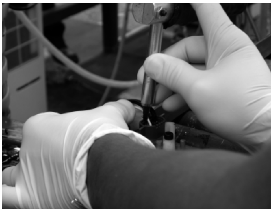
Potting/sealing of sockets. Empire Electronics is the leading supplier in the automotive lighting arena for potted sockets.
