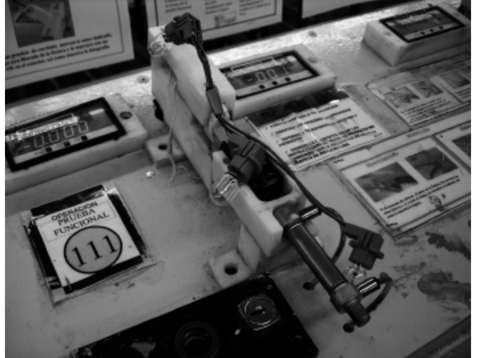
Continuity testing is a critical part of Empire's "quality net" area.
