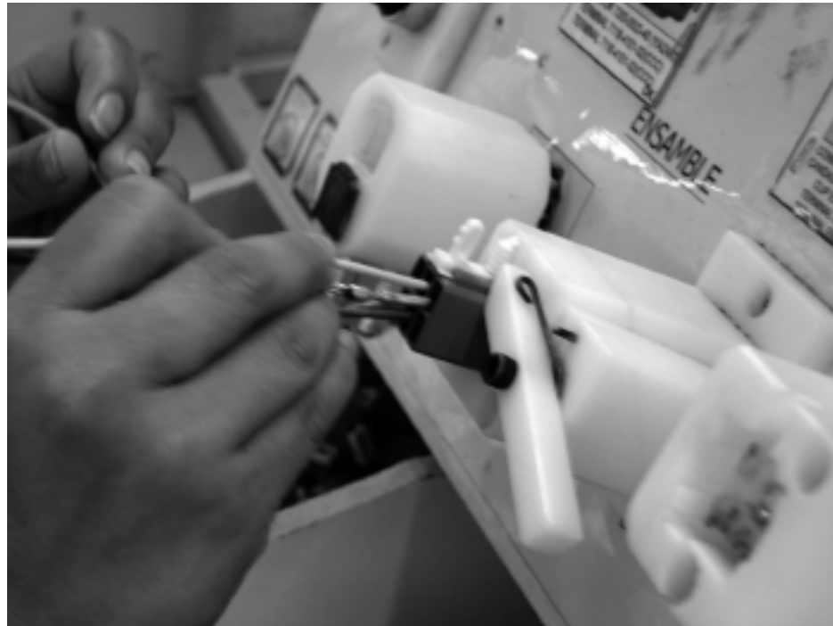
Connectors are placed in testing fixtures during assembly. This is an example of a poke yoke system.
